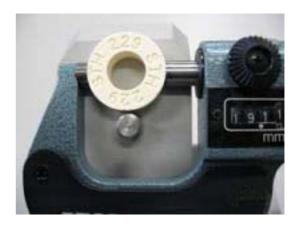
The "T"'s impressed in the ring should be placed exactly on the indentation of the micrometer.
